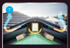
Remove the release paper from the adhesive butyl on one side, and stretch the flashing slightly at the top to facilitate air flow and stick down. Repeat on other side. The flashing should be stretched away from the ridge, towards the eaves. This will open the breathable membrane in the centre of the flashing and allow maximum ventilation.
