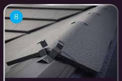
At the gable end, use 30mm galvanised wood screws to fix the first RapidRidge Clip to the centre of the ridge batten. Insert the ridge cap centrally on the ridge batten into the fold of the clip. With the first ridge cap in place, fix the 2nd clip on top of it at the other end to fix the ridge cap securely in place.
